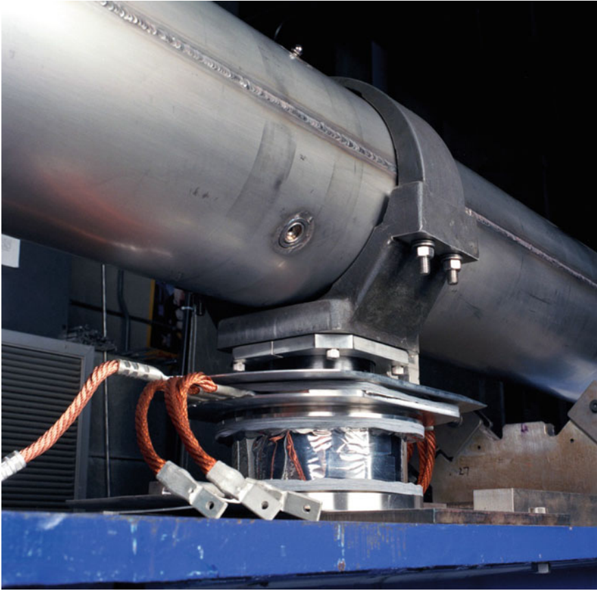
Fig. 2.9 Cold mass and cradle and support post assembly
