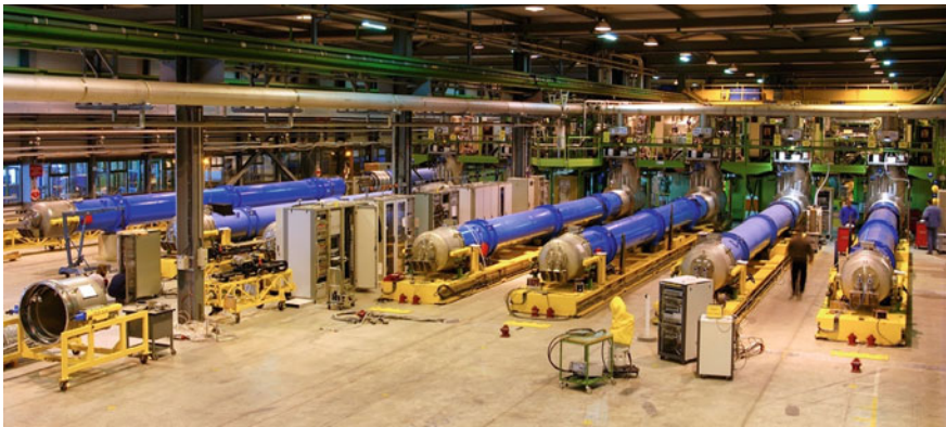
Fig. 3.18 Cryogenic tests of magnets at CERN (CERN photo)
