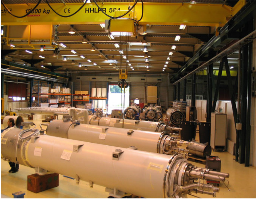
Fig. 3.16 Short-straight-section cryostat assembly hall (CERN photo)
