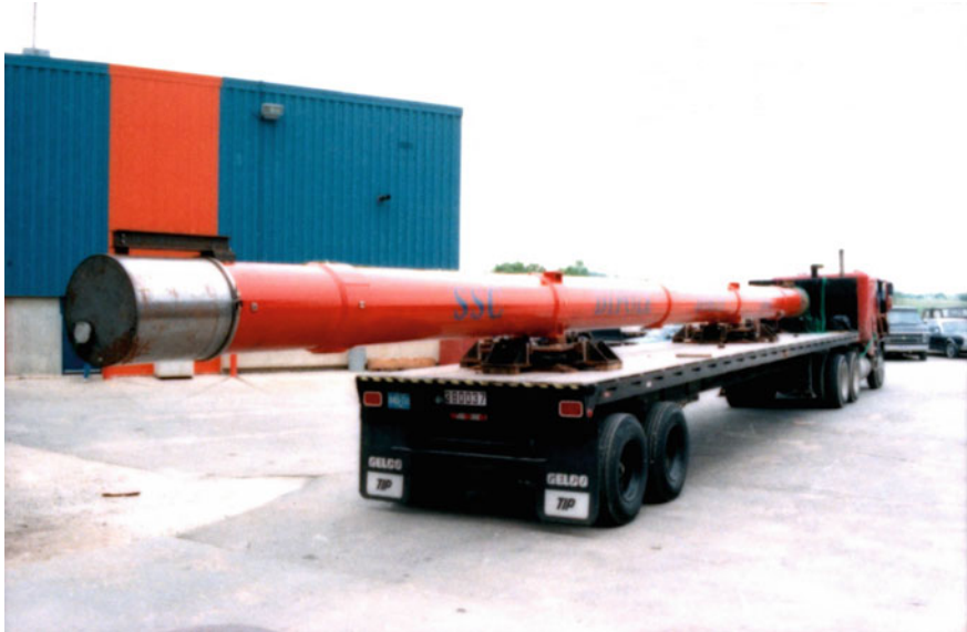
Fig. 2.3 SSC 50 mm collider dipole complete magnet
