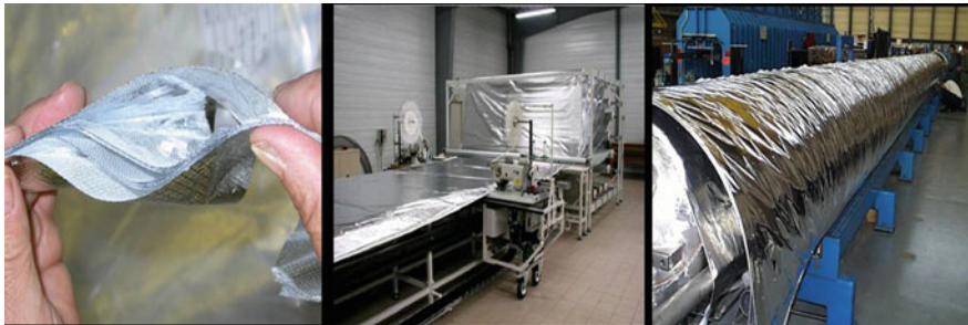
Fig. 1.8 The MLI system for the large hadron collider (LHC) magnet cryostats. Reproduced with permission from Poncet and Parma [16]. Copyright 2008, AIP Publishing LLC
