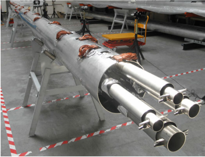
Fig. 9.23 Aluminium thermal shield of the XATL1 straight module with its copper thermal links to the thermal shield return line ( courtesy Kriosystem Ltd.)
