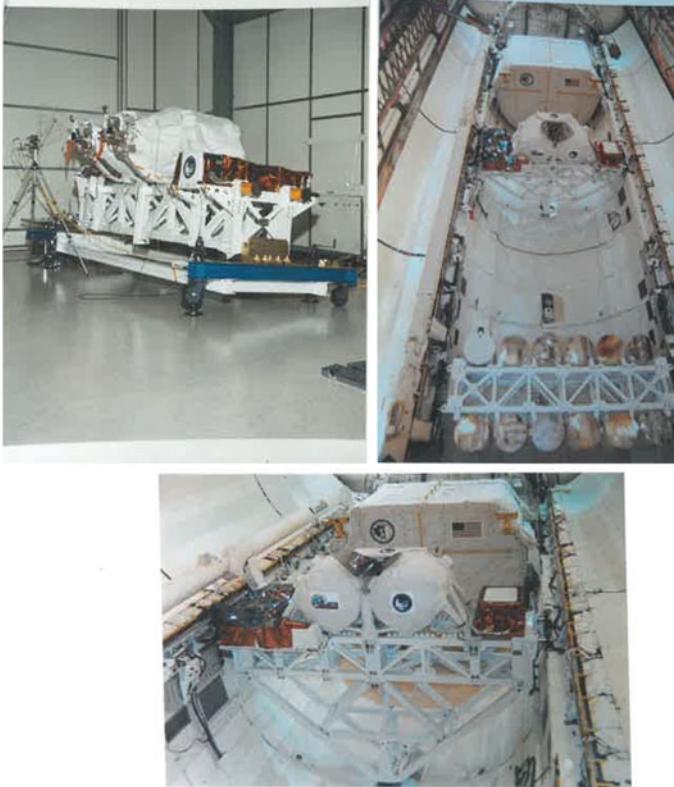
Fig. 4.4 SHOOT at Kennedy space center. Upper left SHOOT on the cross bay bridge. Upper right SHOOT mounted in STS-57. Lower center SHOOT is mounted near the top of the payload bay just behind the Spacehab module
