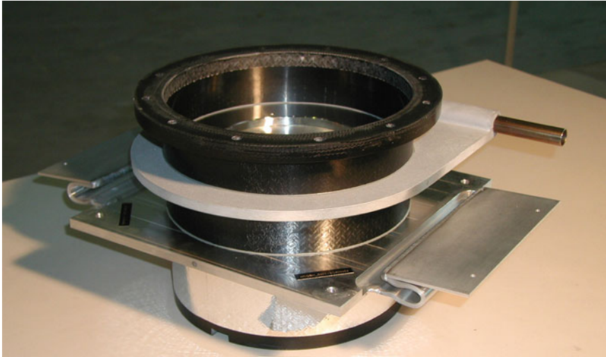
Fig. 3.14 Glassfibre-reinforced epoxy support post (CERN photo)
