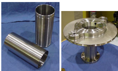
Fig. 6.16 He gas cooling passages ( right ) and FPC outer conductor assembly ( left ). The helium gas flow rate of 0.038 g/s produces an exhaust temperature of 210 K ( center )
