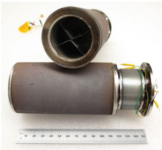
Fig. 4.5 Picture of two high-flow phase separators. The cylinders are made of porous sintered stainless steel in a reentrant geometry to maximize the flow area and minimize pressure drop across this device
