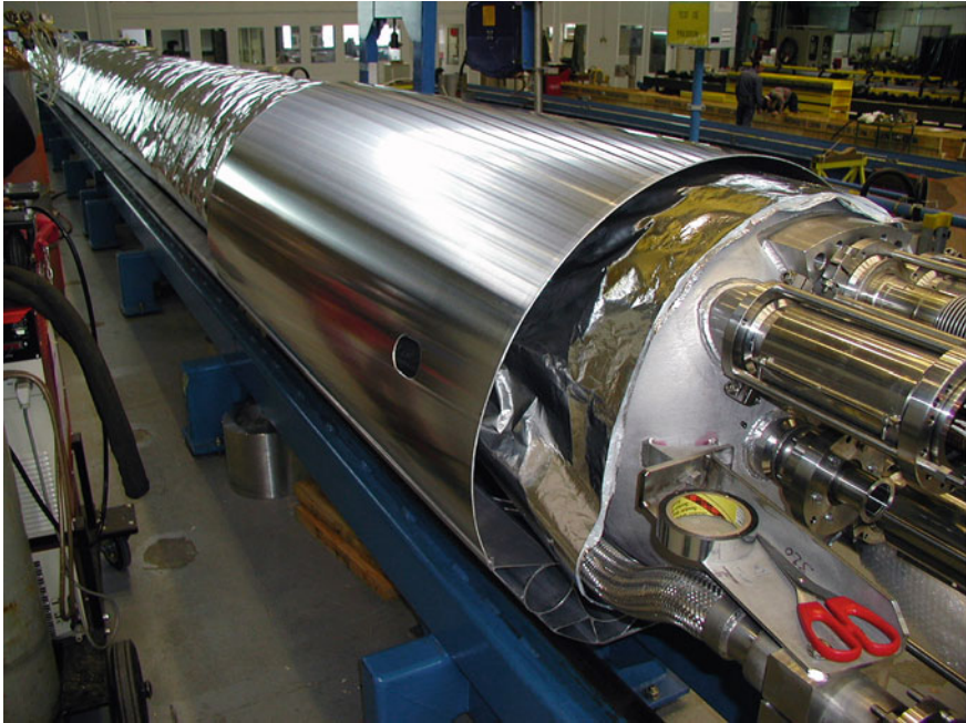
Fig. 3.11 Aluminium A1100 shell of cryostat thermal shield (CERN photo)
