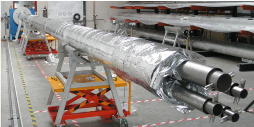
Fig. 9.24 MLI radiation foils wrapped on the XATL1 straight module thermal shield ( courtesy Kriosystem Ltd.)
